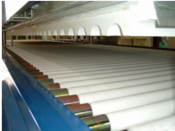
**Fused Silica Rollers with heat resistance metal shaft for metal processing**
